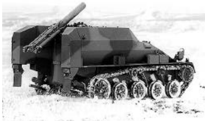
Figure 13 The Wiesel mortar variant is an example of the family of air-transportable armored fighting vehicles armed with precision weapons available to equip the initial Precision Maneuver rapid reaction corps. MAK System Gesellschaft MBH - Light Airtransportable Armoured Systems [WWW page] (The Website for Defence Industries - Army, 2000 [cited 26 March 2000]); available from http://www.army-technonology.com/contractors/armoured/mak/index.html .
