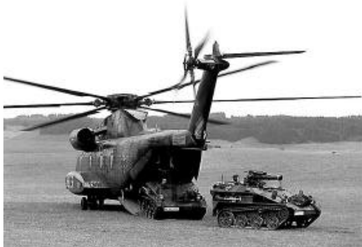
Figure 7 German Army Wieselo TOW Carriers unload from a CH-53 Helicopter. MAK System Gesellschaft MBH - Light Airtransportable Armoured Systems [WWW page] (The Website for Defence Industries - Army, 2000 [cited 26 March 2000]); available from http://www.army-technonology.com/contractors/armoured/mak/index.html .
